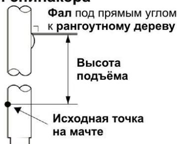
(l) **ВЫСОТА ПОДЪЁМА СПИНАКЕРА [SPINNAKER HOIST HEIGHT]\***
